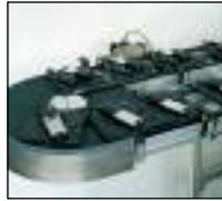
automotive parts assembly where plant floor space is a premium. Steel, aluminum, and economical plastic pallets are available. All pallets have a locating detent for precise positioning.
